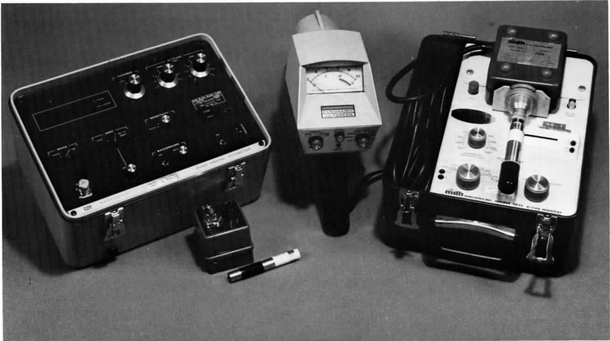
Figure 2.4. Radiation measurement equipment. The survey meter (*center*) is not suitable for dosimetry or QC purposes. A pen dosimeter, shown in the lower left with its charger-reader, can be used for limited purposes, but because of its inherent limitations we do not feel it is accurate enough for QC purposes. Direct readout dosimeters (*on the left and right*), although somewhat costly, are essential for reliable and accurate dosimetry and for a good QC program.
