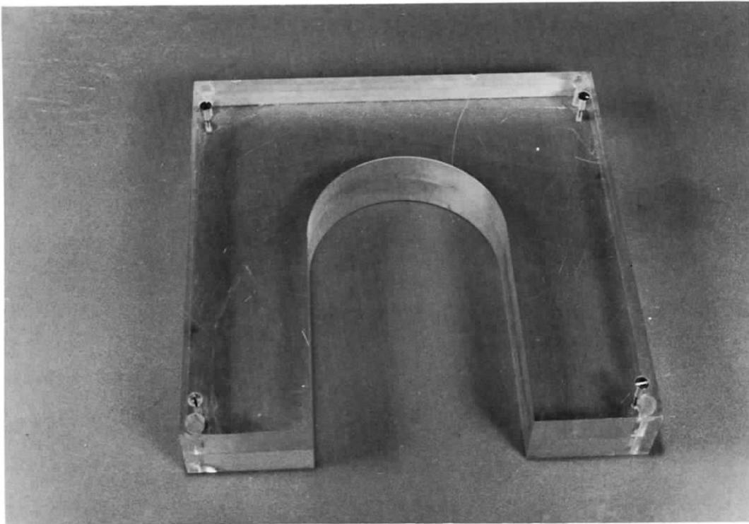
Figure 2.1c. Base for the PEP, which is used when dosimeter readings are to be made under the phantom.
