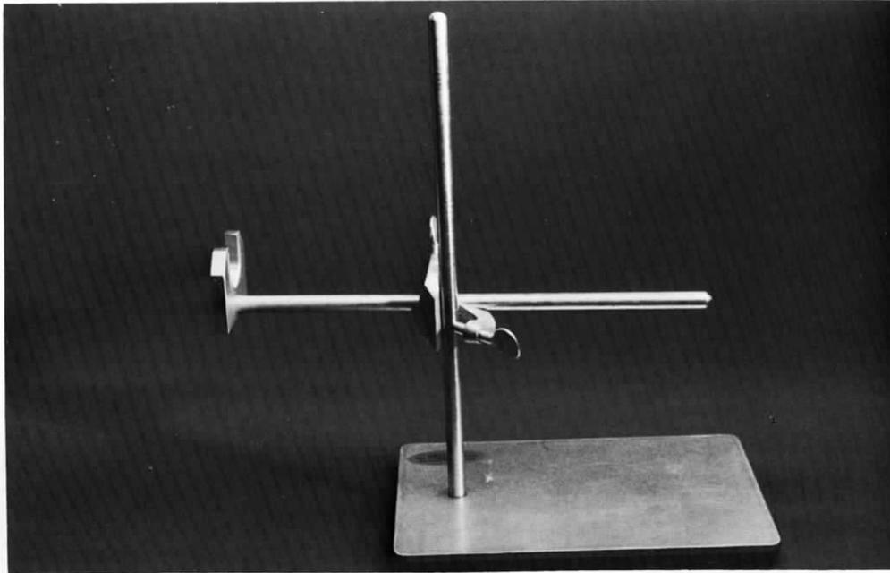
Figure 2.5b. Although not essential, a stand can be constructed with a lead-weighted base to hold the dosimeter at the appropriate level for measurements.
