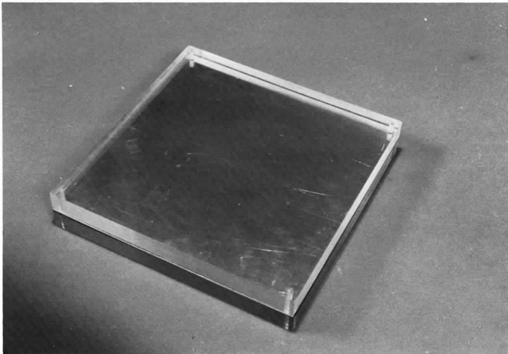
Figure 2.2b. The extremity phantom consists of a 2-mm sheet of type 1100 aluminum sandwiched between two 1-inch (2.5-cm) sheets of acrylic.
