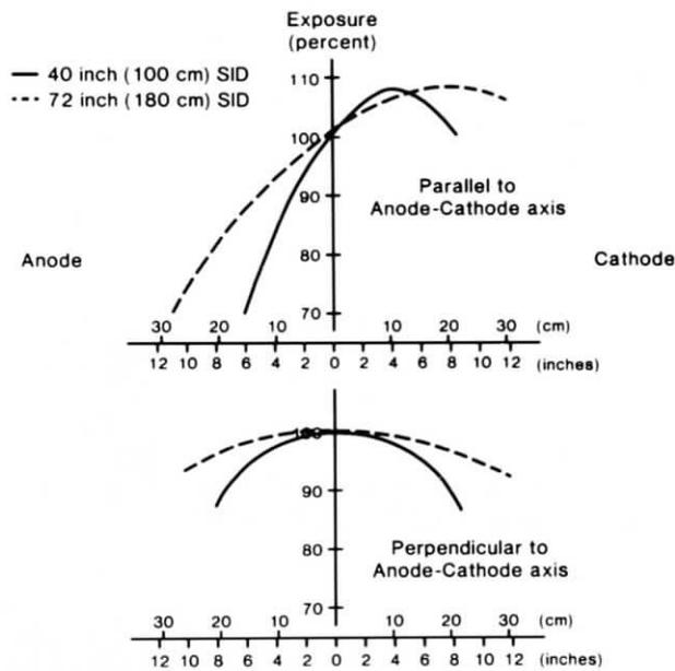
Figure 2.8. The heel effect can cause difficulty in making radiation measurements. Considerable variability will be noted as the ionization chamber is moved parallel to the anode-cathode axis, especially with a 40-inch (100-cm) SID. Variation is not nearly as significant perpendicular to the anode-cathode axis, but it is still present.
