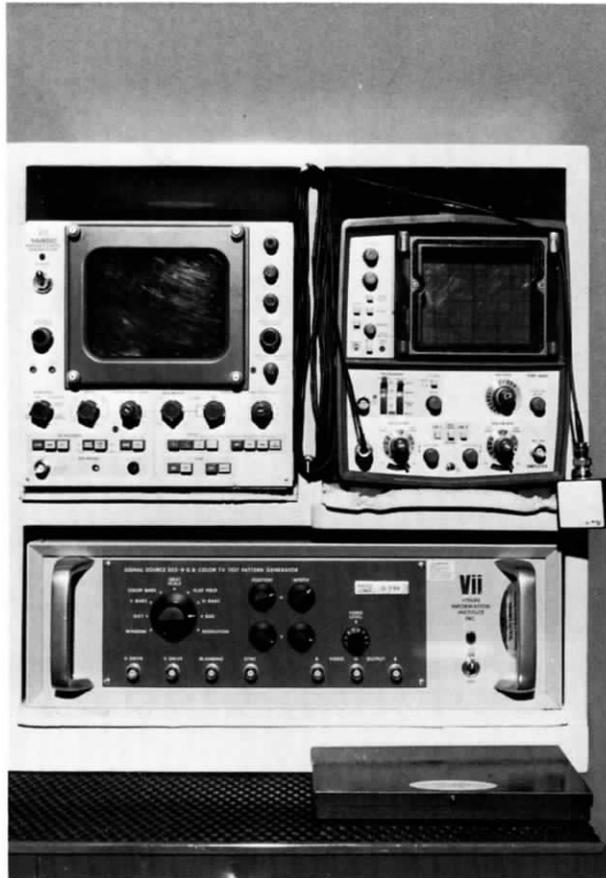
Figure 2.6c. Electronic test equipment includes a video waveform monitor (*upper left*), a storage oscilloscope with a solid-state detector connected to it (*upper right*), and a video signal generator (*bottom*), all sitting on foam (for shock absorption) in a specially designed cabinet. Note also the lead letter and number identification kit on the lower right.
