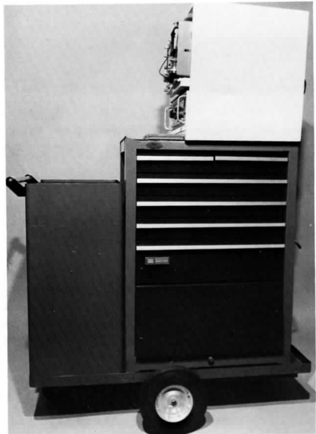
Figure 2.6b. All QC test tools are contained in the locked drawers and lower storage area (including the PEP). One small drawer is lead-lined so that film can be stored in the cart without risking film fog. The flat area to the left provides a writing area. Various ionization chambers are stored in one drawer, which has been lined with foam containing cutouts to fit each chamber.
