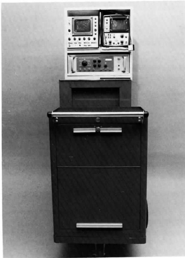
Figure 2.6a. Quality control equipment cart. It is convenient to have all of your equipment on one cart so that it is available when you are working in a room. The locked section contains tools (screwdrivers, pliers, etc.) and the readout section of the dosimeter. The rack on top was added to the cart to hold electronic test gear.
